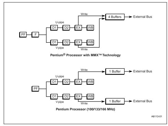
Figure 16-10. Embedded Pentium® Processor Write Buffer Implementation
